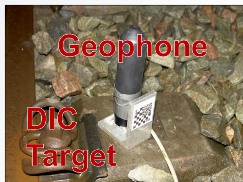
Figure 3 – Geophone and DIC target
