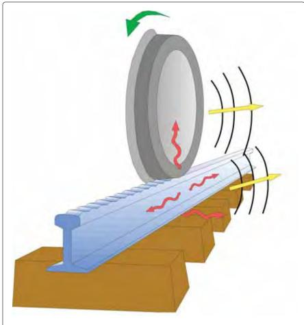
Figure 1: Schematic diagram of the process of generation of rolling noise
