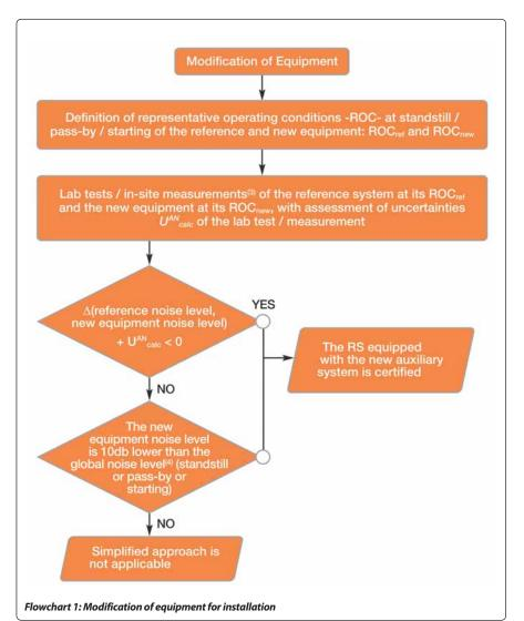
applying the TSI Noise; the type of rolling stock to which the method is applicable has to be specified case by case.
