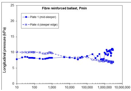
Fibre length/width/thickness: 300mm/100mm/0.5mm
